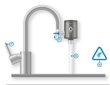
• We recommend to mount the Alb Filter® DUO on the right side or aligned to the front to make the switchover function (filtered/unfiltered) easier to operate.
